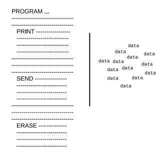
But with object-oriented programming, it is the data that is modularized. And each data module includes its own operations for performing actions directly related to its data.
